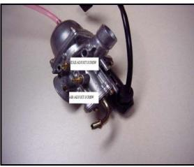
Air/Fuel Ratio adjusting procedure:
