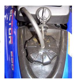
hole while operating the unit. The fuel cap vent and vent tube must be clean and clear of obstructions for the unit to operate normally. You can check the vent and vent tube by blowing air through the tube. If you can not blow through the vent tube and cap you must clean the vent and tube or replace them.
