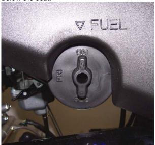
The valve has three settings; "PRI", "ON" and "RES". With the valve in the "ON" or "RES" position fuel flow is controlled by a vacuum vale in the petcock. Fuel will begin flowing to the carburetor as soon as the engine is turned over. "ON" is the normal operation position of the fuel valve. When you have to switch to the "RES" position you must refuel the unit as soon as possible to prevent running out of fuel.
