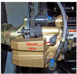
brake system must be purged of air in the lines and reservoir.
