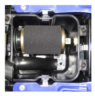
To maintain the highest performance from your engine and to reduce excessive wear that could cause engine failure the engine requires a continuous flow of clean air. Air is taken into the engine through an air filter to clean the air prior to mixing it with fuel and oil in the carburetor.
