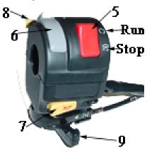
The stop switch is a red colored rocker switch located on the left-hand handle bar.
