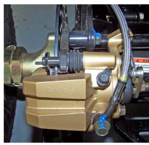
Visually inspect the brake hose for any signs of wear or leaks.
