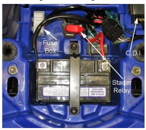
Do not expose the battery, for extended periods of time, to freezing temperatures. If the battery has been frozen it will need to be replaced. There is an inline fuse on the positive lead of the battery to protect the wiring system from over loads. If your starter motor will not turn over and the battery is fully charged, check the inline fuse on the unit.
