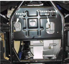
The Vector 250 requires SAE85W-140 gear oil to lubricate and cool the transmission and drive gears. Transmission oil level should be checked before each riding session and change
