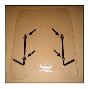
**STEP 1**—Loosely mount the two support bars onto the windshield using the hardware layout shown above.
