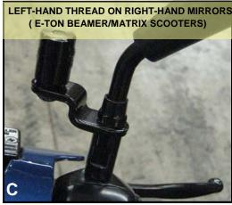
**STEP 2**—Remove the mirrors by using a 14mm wrench and unscrewing them. Assemble the support arm bracket to the window barrel mount using the star washers and Allen head bolts as shown in (A).
