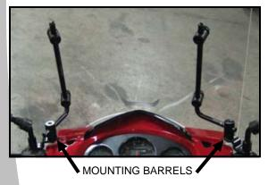
**STEP 3**—Take the windshield assembly and slide the lower ends of the support arms into the mounting barrels attached near the mirrors as shown in the picture.
