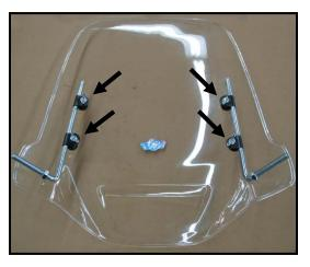
**STEP 1**—Loosely mount the two support bars onto the windshield using the hardware layout shown above.
