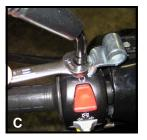
STEP 2—Remove the mirrors by using a 14mm wrench and unscrewing them, then center the arm support bracket over the threaded mounting hole on the handlebar (A). Then, reattach the mirror through the hole in the support bracket (B, C).
