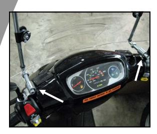
**STEP 3**—Take the windshield assembly and slide the lower ends of the support arms into the arm brackets attached below the mirrors as shown in the picture.
